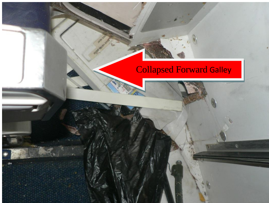
Photo 5. View of Collapsed Forward Galley
